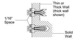
Figure 8 - Tightening Anchors
